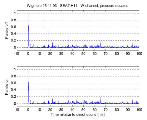
Figure 7: Pressure squared time response with and without the laylight panel, measured in a specularly covered seat. The reflection at 37 ms corresponds to the ceiling reflection and is mildly stronger in the case with the panels in place.
