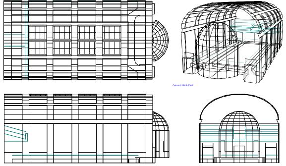
Figure 1: Plan, sections and 3D wireframe model of the Wigmore Hall. (In reality, the concave surfaces are continuous and not facetted as shown here.)
