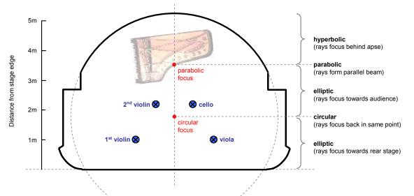
Figure 5: Plan of the stage platform at Wigmore Hall, showing typical locations of a string quartet and a grand piano. The different zones and points of hyperbolic, parabolic, elliptic and circular reflective behaviour from the apse are also identified.
