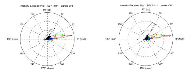
Figure 8: Elevation of the instantaneous sound intensity (on a linear scale to only show the strongest reflections), with and without the panels. The colours correspond to the reflection arrival time (red = 0.10 ms, green = 10.20 ms, blue = 20.30 ms, black = 30.40ms). The red loop corresponds to the direct sound, the green loop to a strong side wall reflection and the black loop to the ceiling reflection. The ceiling reflection is clearly stronger when the laylight panels are in place.
