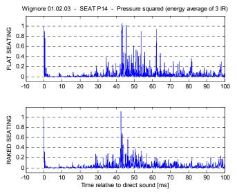
Figure 9: Influence on a room impulse response from putting the 9 rear seating rows on a subtle rake. The strong reflections at 45 ms, 54 ms and 62 ms diminish by raising the rear seats.
