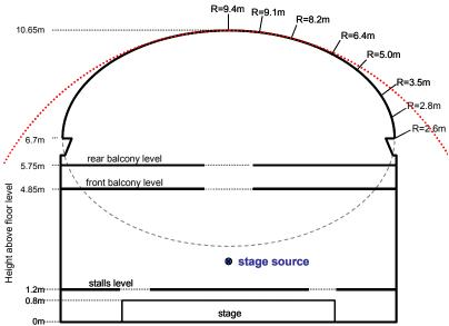
Figure 3: Cross section showing the elliptic ceiling. The numbers indicated along the ceiling represent the local radius of curvature (R). The red dotted line is a circular approximation of the top part, with radius 9.4 m.
