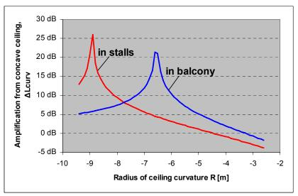
Figure 4: Theoretical amplification (in dB) from the concave ceiling as a function of the varying radius of curvature, for a source at 1.4m above the stage floor.
