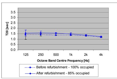
Figure 10: Reverberation time before and after the 2003-2004 refurbishment, in the occupied condition.
